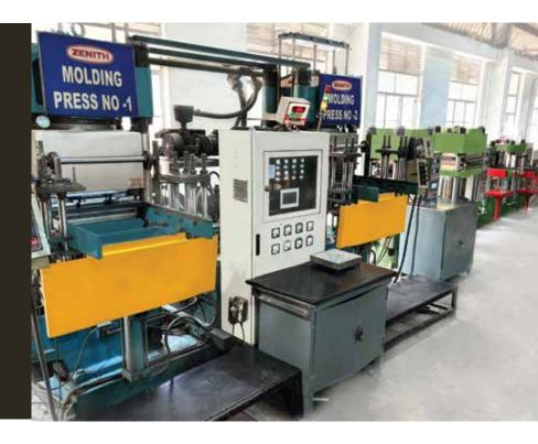
Zenith Manufactures wide range of custom rubber molded products in polymers like EPDM, NBR, CHLOROPRENE, SILICONE, FLURO SILICON, FKM, ACM, AEM (VAMAC), SBR, NATURAL RUBBER. We produce molded products by using compression molding, transfer-molding process. Special controlled processes are developed by Zenith to produce such high performance molding products.
